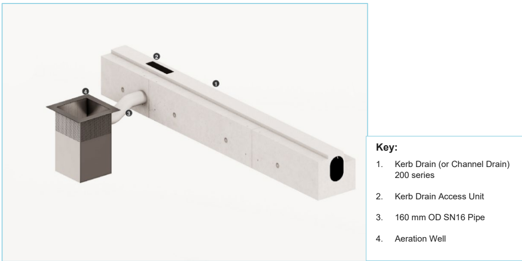
Figure 8: Inlet system components
