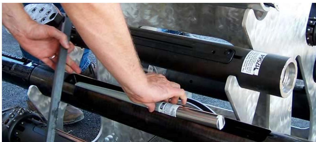
FIGURE 4.5: GENERAL EXAMPLE OF A TRANSMITTER PLACED IN DRILLING PIPE (Picture Courtesy Of Digital Control Incorporated)
