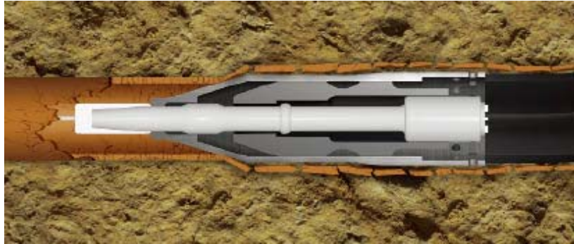
FIGURE 6.4: EXAMPLE OF AN HYDRAULIC BURSTING HEAD (Graphic Courtesy of Miller Pipelines)
