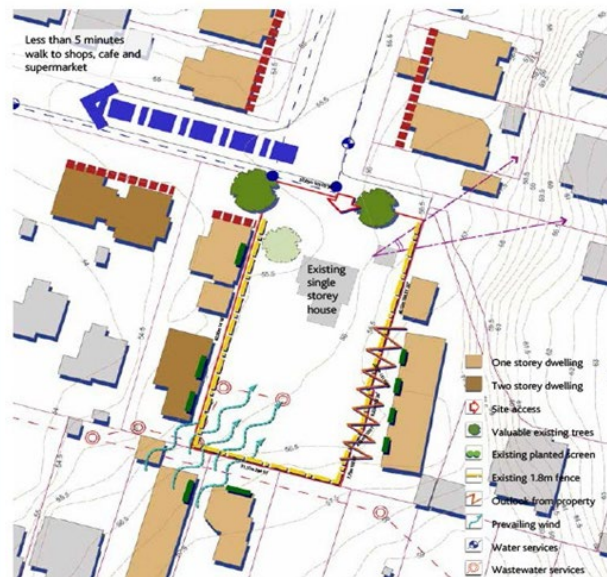
An example of a site analysis plan identifying the natural and built characteristics of the site
