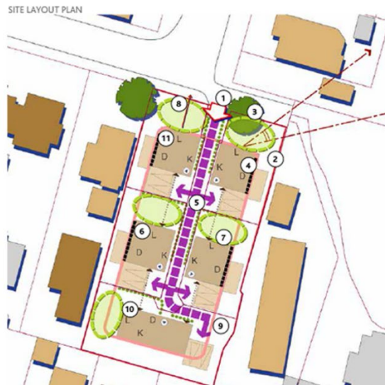
Concept plan illustrating design principles through a simple diagrammatic drawing
