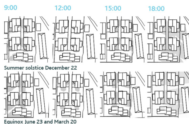
Shadow diagrams showing sunlight access and shadowing at different times of the day and year.
