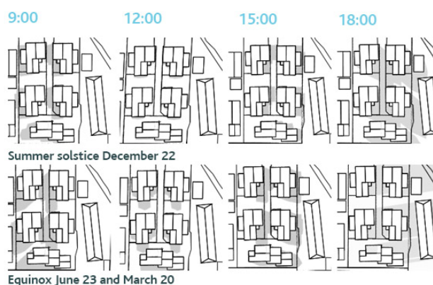
Collection of maps showing sunlight access and shadowing at different times of the day and year
