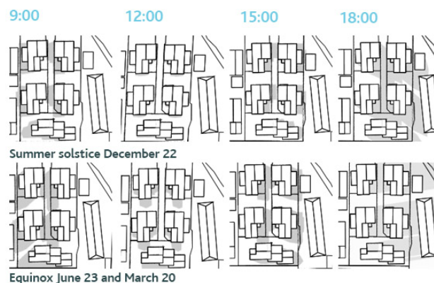
Collection of maps showing sunlight access and shadowing at different times of the day and year
