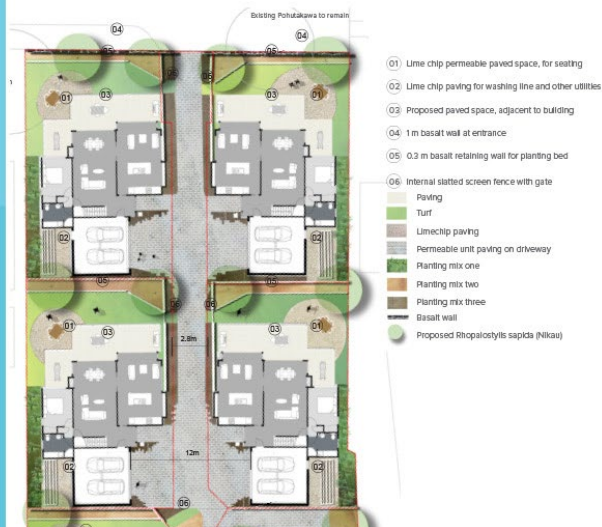
Landscape plan illustrating soft and hard landscaping around the proposed built elements
