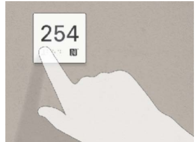
Tactile embossed and braille coded UAP marker (Sourced from CMHR, Ian McCausland).
